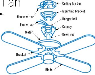
7. Attach the blades: Attach the blades to the motor housing using the included screws and a screwdriver.
